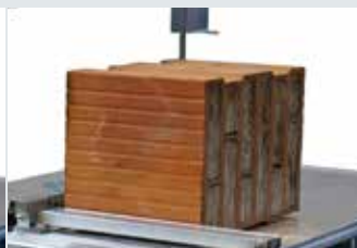
Perlite filled porous brick
