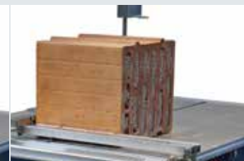
Mineral wool filled porous brick
